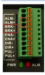
To operate the motor, the brake must be supplied with 24V. If the brake is not supplied with the correct voltage (24V) and sufficient current (150mA), it is fixed. It is strongly recommended not to operate the motor with the brake fixed, as the increased current consumption can damage the electronics.
