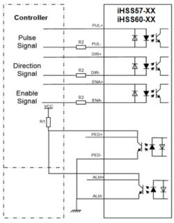
$\begin{array}{ll} \mbox{VCC} = 5\mbox{VC} & \mbox{R2} = 0\mbox{\Omega} \\ \mbox{VCC} = 24\mbox{V} & \mbox{R2} = 1\mbox{k}\mbox{\Omega} \sim 1,5\mbox{ k}\mbox{\Omega} \end{array}$
