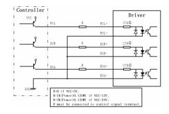
Figure 4: Connection to PNP signal (common-cathode)
