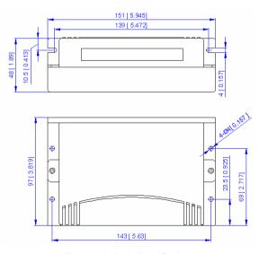
Figure 1: Mechanical specifications
