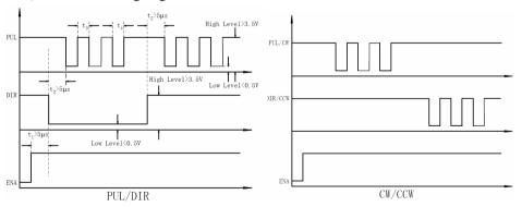
Figure 11: Sequence chart of control signals
