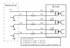
Figure 3: Connections to open-collector signal (common-anode)
