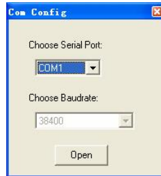
Figure 21: RS232 communication configuration window
