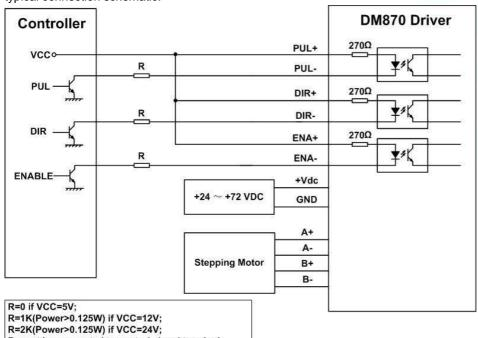
R must be connected to control signal terminal.
