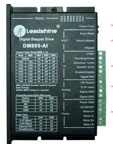
Indicator Green: Power, Red: Fault Potentiometers Adjusting Speed, Acceleration, Deceleration Digital I/O Signal Connector, 6-pin screw terminal, 3.81 mm Analog Signal Connector, 6-pin screw terminal, 3.81 mm Power Connector, 6-pin screw terminal, 3.81 mm space
