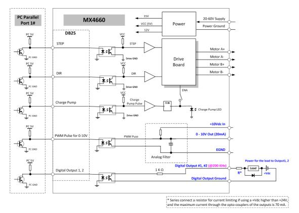
Figure 16 Connecting digital output1, 2
