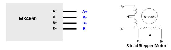
Figure 8 Connecting an 8-lead stepper motor in series connection
