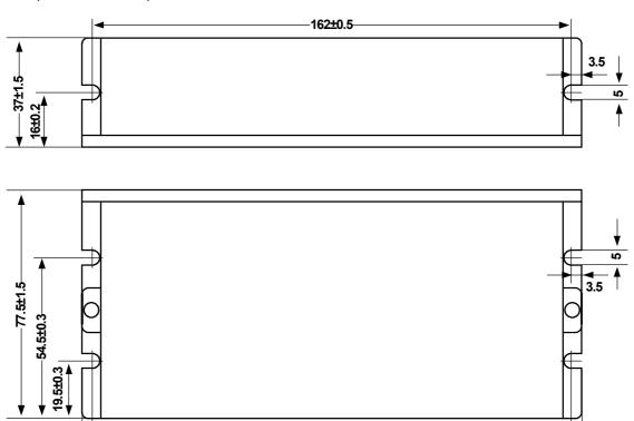
Figure 1 MX3660 mechanical dimensions
