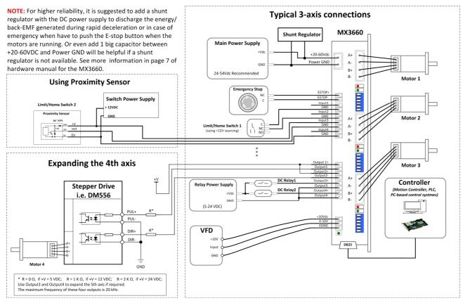
Figure 6 MX3660 connection diagram
