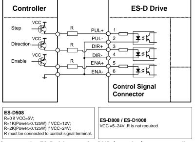
Connect the ES-D drives to the PNP (sourcing) type controllers
