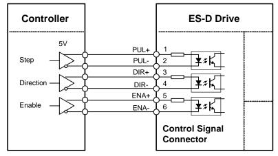
Connect the ES-D drives to differential type controllers
