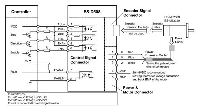
Typical connections of the ES-D508 with controller of sinking output
