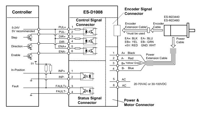
Typical Connections of the ES-D1008 with controller of sinking output
