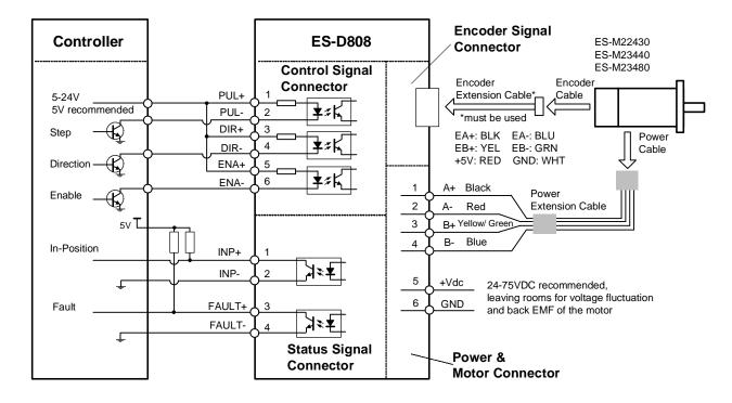
Typical connections of the ES-D808 with controller of sinking output
