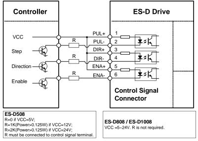
Connect the ES-D drives to the NPN (sinking) type controllers
