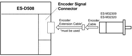
Encoder connections between the ES-D508 and ES-M3 series motors
