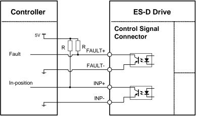
Fault, in-position signal connection of the ES-D drive (Note: The ES-D508 does not have in-position output)
